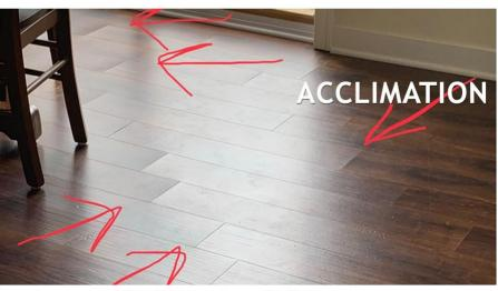
Allow boxes of flooring to acclimate for 24 hours in room temperature. SPC flooring has the least expansion rate of any vinyl flooring. But extreame changes in temperature can lead to small expansion. Thats why its still a good idea to install your flooring once it has acclimated to room temperature.
